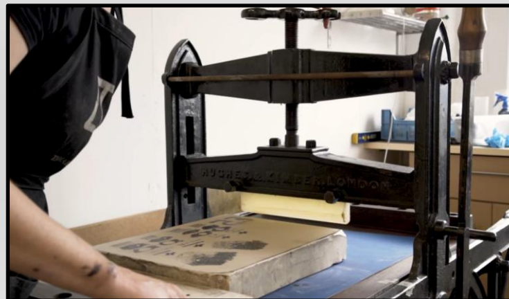
Imprinting the image while pushing stone under pressure
