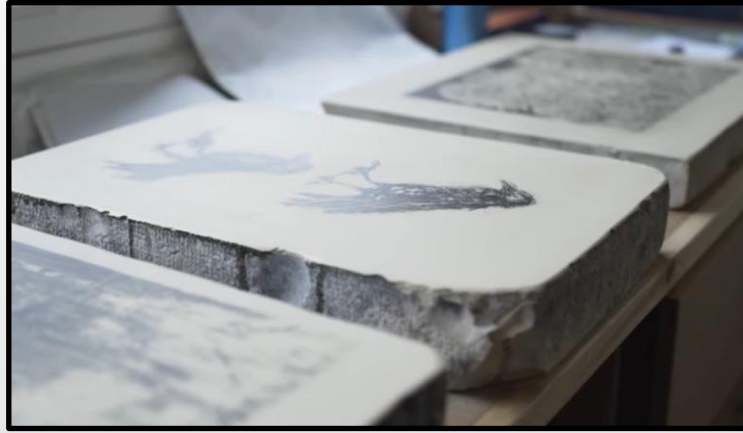
Drawing image with grease pencil in reverse
