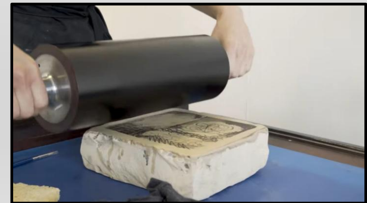
Inking with leather roller, after washing with solvent
